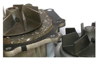
Image 1: Displaced impeller with scoring (left); correct position of the impeller (right)
